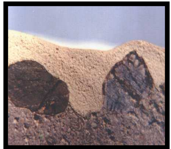
Close-up cross-sectional view of ECOSYSTEM® Expanded coating.
